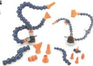
cutting fluids, polishing liquids or cleaning fluids. FH hoses are available in  $\frac{1}{4}$  in or  $\frac{1}{2}$  in bore sizes with matching components and are easily shortened or extended as each segment clips together to ensure liquids can be easily, quickly and accurately directed exactly where needed. They are suitable for a maximum input pressure of 4 bar.
